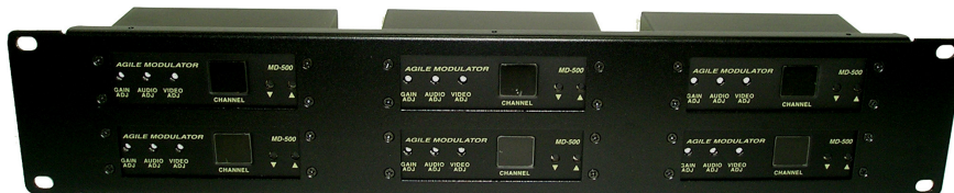
Black 2U 19 inches with 6 ones, hold modulator, demodulator or video distributor.
